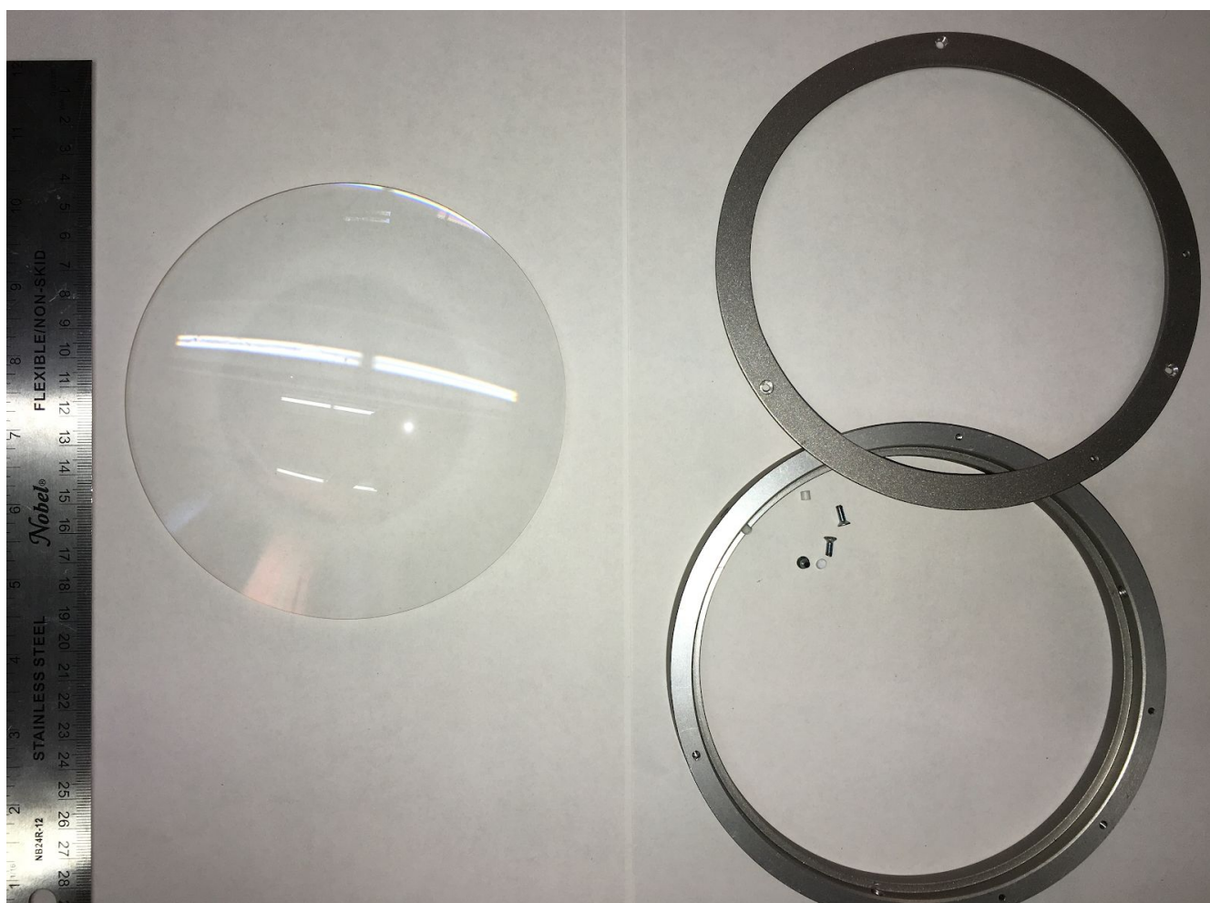
150mm Dia x 300mm Focal Length, PCX Condenser Lens ( www.edmundoptics.com Stock #27-509)
