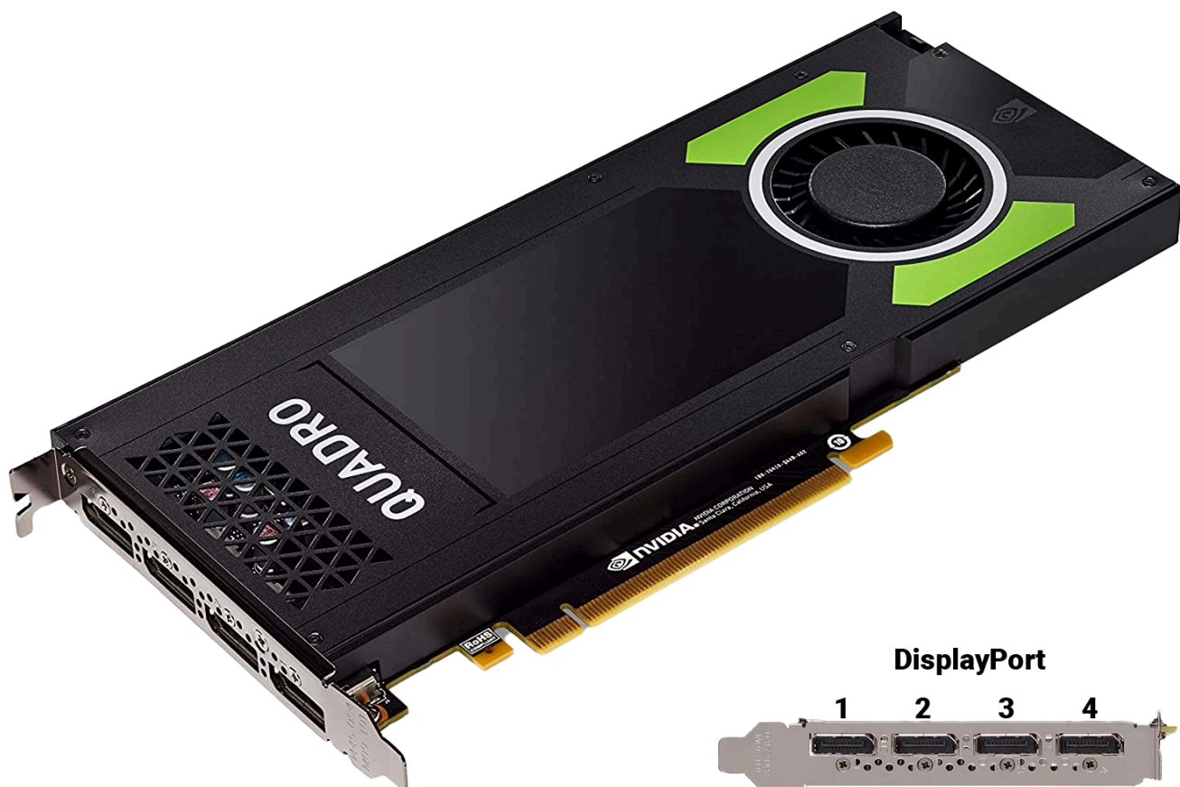
nVidia Quadro P4000 w/ DisplayPort layout
