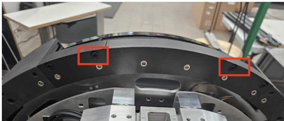
Drum with nylon screws highlighted.
