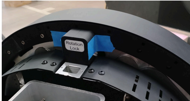
Rotation lock taped in place.
