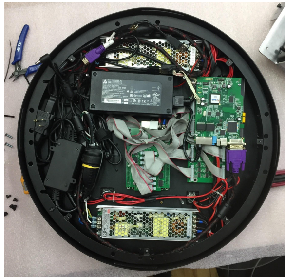
Underside of display without bracket and computer (the PCB referenced above is on the right with the purple HDMI-DVI cable)
