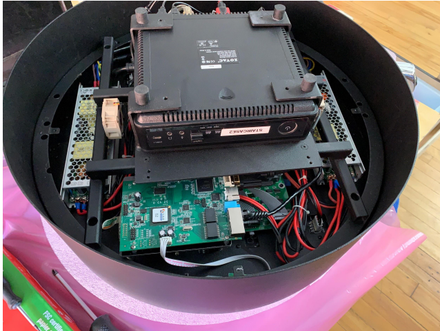
Underside of display with computer
