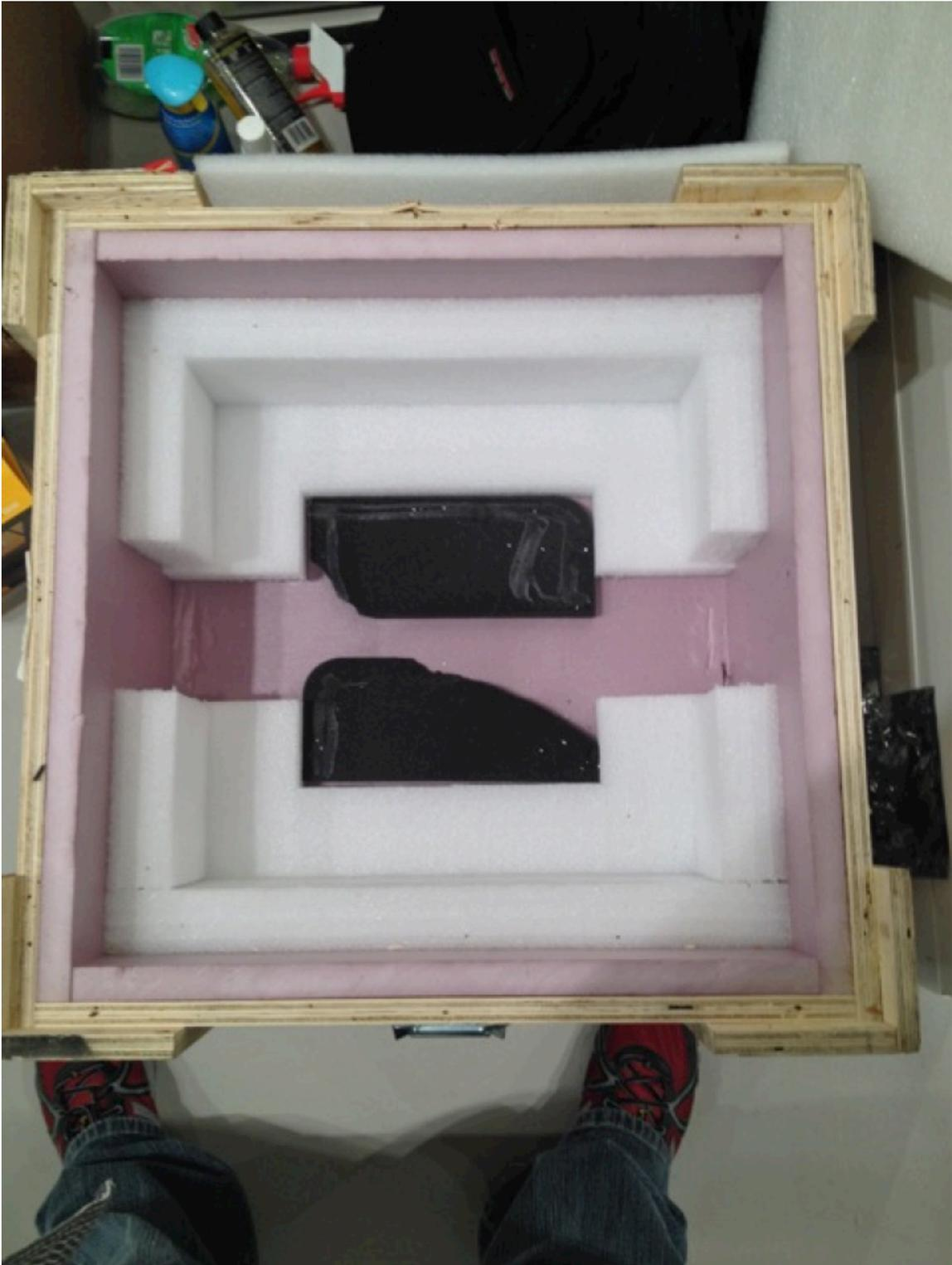
Lay down the white styrofoam pad on top of the 2 gray foam pads (if you had no gray foam pad, the white styrofoam should have some foam glued on in order to make it thicker). Once we have the white styrofoam pad in place, the zone covered with the pad should be slightly higher (around 0,5 centimeters) than the zone not covered. This will prevent the monitor to bend and break during shipping.
