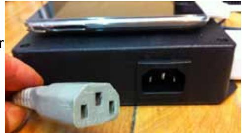
You can ONLY connect the piece to 100-120V 60Hz (American) or use with a step-down converter in regions that have 210-240V 50Hz (European). Unless we specifically manufactured a copy that can natively run on 210-240V without a converter.
