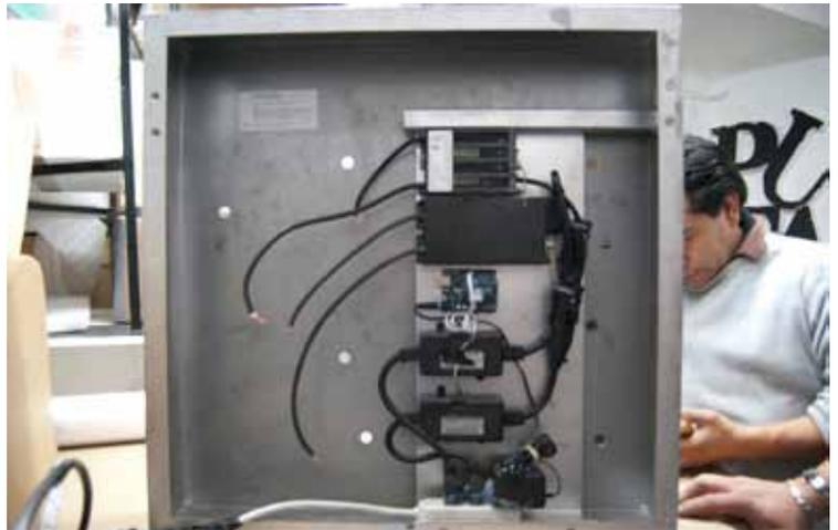
The two remaining ends for the top two words need to be connected to one ballast and the other two words to the second ballast. Again, connect the wires by twisting them.
