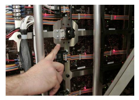
3. Make sure the main controller board is still in place. With the pins on the left well connected and the board well screwed.
